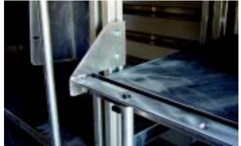
Adjustable retainer guide allows cola bays to be adjusted for more snack space when necessary
