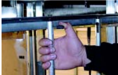
"Quick Release" thumb latch retainer bar can be engaged with slight thumb pressure
