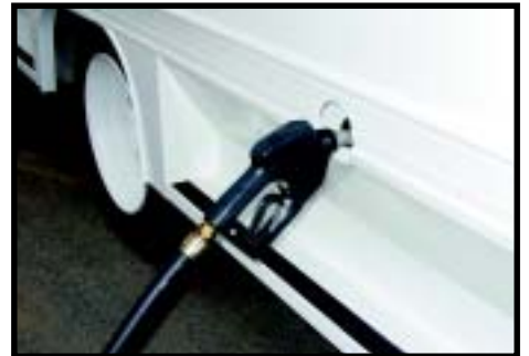
Fuel tank filler spout located on outside of body to optimize inside space
