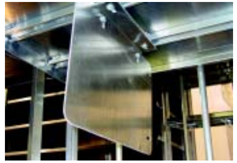
20-oz. soft drink bays can be converted for 12-oz. cans by a simple shelving adjustment.
