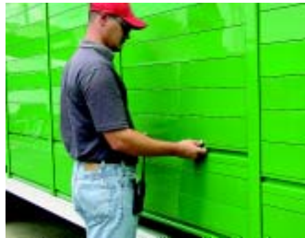
Roll-Up door with intermediate handle panel for safe easy operation
